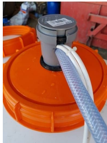
standpipe mounted in the cap
